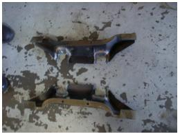
2. Remove the exhaust system and cut away the spare wheel holder to create room for the LPG cylinder.
