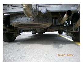
1. This cylinder is designed to be mounted underneath the vehicle in the position of the spare wheel, behind the rear differential.
