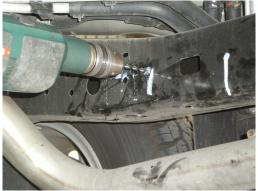
4. Lower the cylinder and drill the marked holes 11mm dia through the chassis. Re-drill the holes on the outer of the chassis 17mm dia to accommodate the crush tubes.
