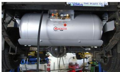
9. Jack the cylinder back up into position and bolt it to the chassis mount brackets fitting the heat shield to the right side bracket. Re-fit the new exhaust system within compliance of AS/NZS1425.
