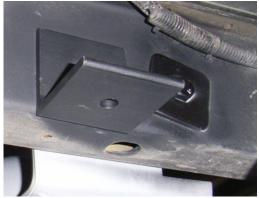
6. Fit the RH chassis mount as previous step but fit the angled exhaust bracket to the outer rear mounting hole as shown. Tighten into position.
