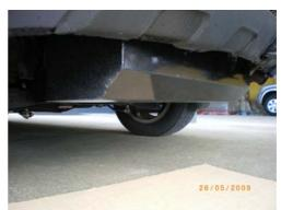
12. Fit the stone / heat protection shield to the cylinder using the bolts supplied. Re-fit exhaust systems with modifications to ensure it does not come within the required distance from the cylinder. (AS/NZS:1425 Clause 3.21).
