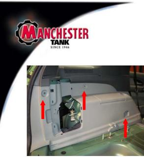
3. Remove the jack assembly and the 3 securing points of the left panel.
