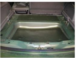
4. With the side panel loose, gently remove the plastic tub from the vehicle.
