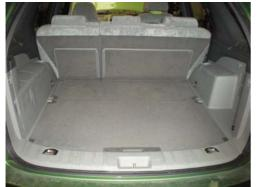
1. Remove the rear floor cover boards (also rear seats if required)
