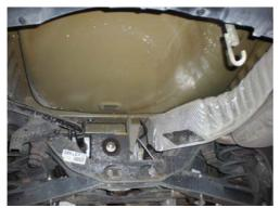
5. Remove the spare wheel and spare wheel securing bracket.
