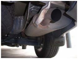
6. Remove the exhaust muffler and tail pipe leading over the rear axle.
