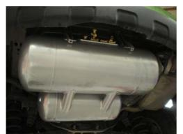
11. Bolt the cylinder into position and re-check the cylinder has maintained clearance from the vehicle.
