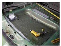
10. Drill the mounting holes using an appropriate size drill bit to suit the countersunk bolts supplied. Mount the cylinder to the vehicle using the backing plates supplied.
