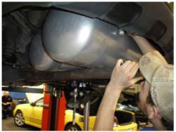
7. Jack the cylinder into position with the valves facing the rear of the vehicle.
